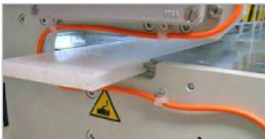
Extraction of the plastic cutting pad on the AF - 1201
